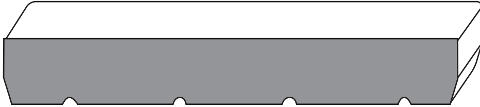
JAMB MC308 1 1/16 X 4 9/16 6' 8" LEGS FJP MC308 1 1/16 X 4 9/16 FJP, MDF, SP, POP, NRO, CH, MP, ALD MC309 1 1/16 X 4 13/16 FJP MC310 1 1/16 X 5 1/4 FJP, SP MC312 1 1/16 X 7 1/4 FJP
