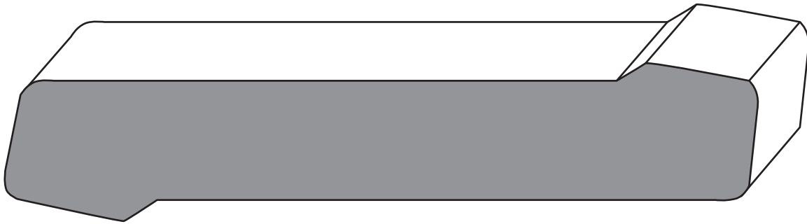
REVERSIBLE SILL MC640 2 X 8 (1 3/8 X 7) TREATED
